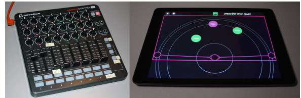
Figure 2: Interface used to represent channel strip metaphor mixing (left) and interface used to represent stage metaphor mixing (right).
