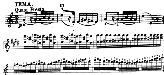
Figure 3: Various situations which cause current staff detection algorithms to behave incorrectly. Top to bottom: “bowing” is possible with a tightly bound book, prominent ledger lines may be detected as part of a staff, and beams may occlude most of the staff.
