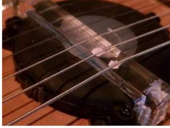
**Figure 2: Feedback Lap Steel Bridge mounted to the Puck tactile transducer**
